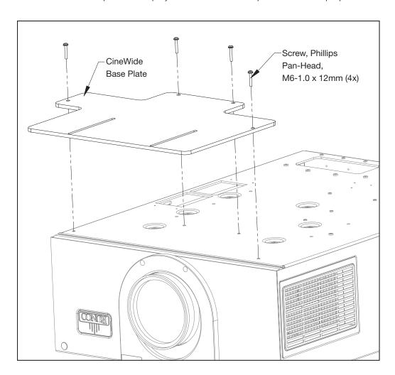
Figure 3-9. Installing the Fixed CineWide Base Plate
